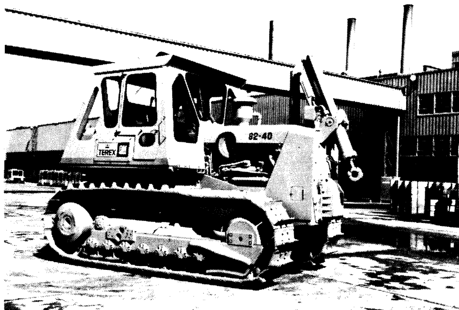
Figure 4-18. Industrial Cab Company ROPS Cab on GM-Terex Crawler
