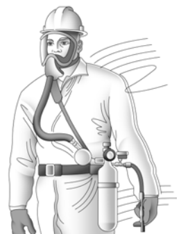
Atmosphere-supplied respirator Full Facepiece Elastomeric with an auxiliary escape bottle APF=10,000 in escape mode only; otherwise APF=1,000 Needs to be fit tested
