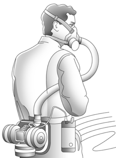
Tight-Fitting Half Facepiece Powered Air-Purifying Respirator (PAPR)
