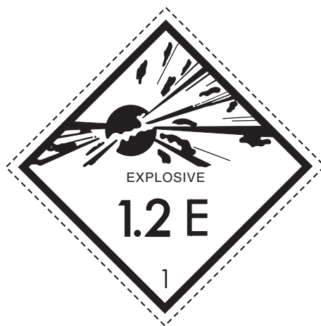
Figure 14.1 Example of label for explosive (Division 1.1, 1.2 or 1.3)
